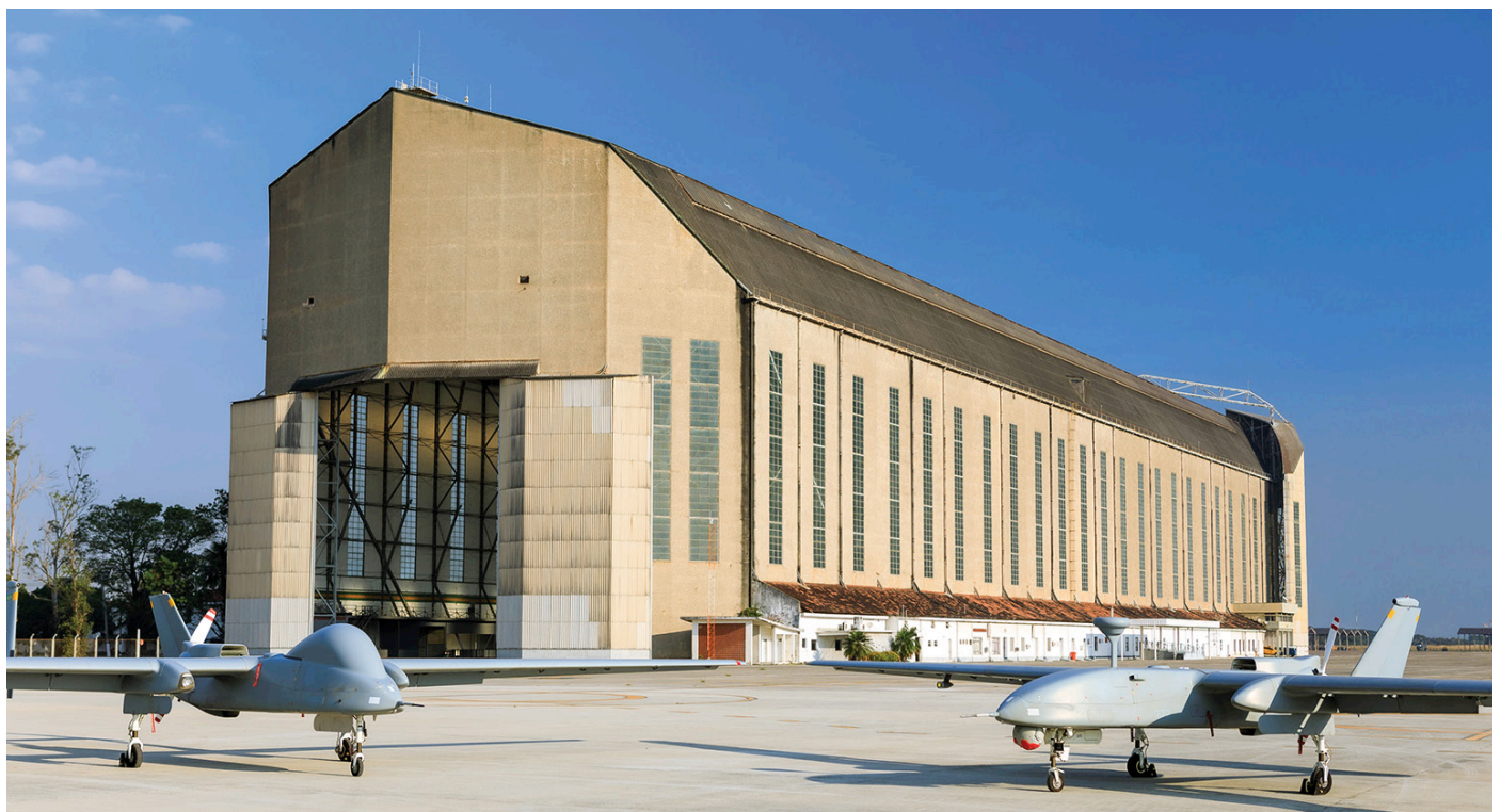
The Brazilian air force RQ-1150 is a VANT. Let us translate that... These machines are 'veículo aéreo não tripulado', or unmanned aerial systems, as we refer to them. Originally delivered as Heron I to the Federal Police and incorporated by 1°/7°Gav to operate along their P-3AM Orions. (Santa Cruz, 23 July 2020, FAB/CECOMSAER Sgt Johnson Barros)
