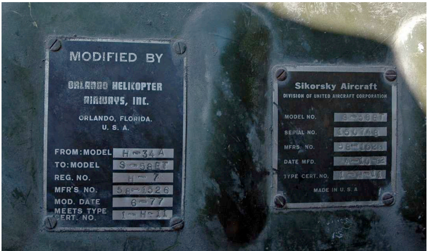
The twin construction number plates of S-58ET H-7 were photographed before the helicopter disappeared from the IDP-camp at the former Bowen Field. To the right is the original Sikorsky plate showing BuNo150748 among other data, and to the left is the plate given by Orlando Helicopter Airways after upgrade to S-58ET, listing Haitian serial number H-7. (03 April 2010, Wim Sonneveld).
